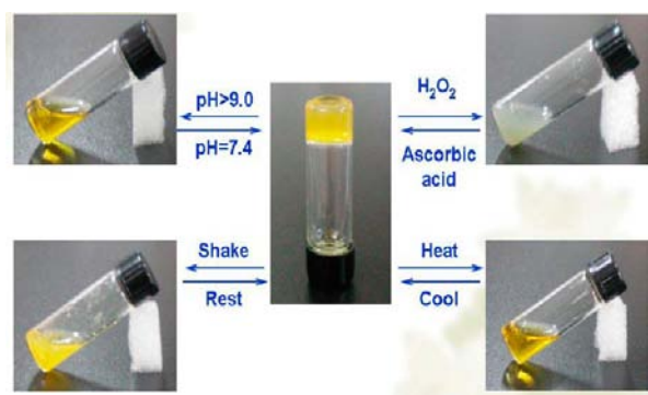
Figure 3. Reversible gel–sol transitions of the supramolecular hydrogel triggered by multiple stimuli (pH, chemical redox reaction, shear stress, and temperature, respectively).
